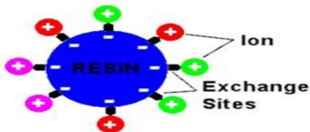
Figure 2. Chemical Structure Of Cation Exchange Resin 7 .
